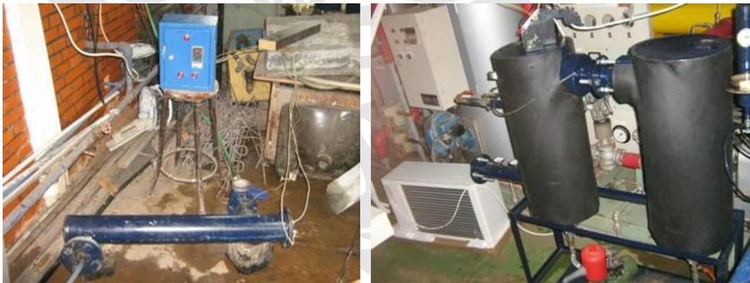
**Gambar 3.4** Alat uji *Throttling Process*
