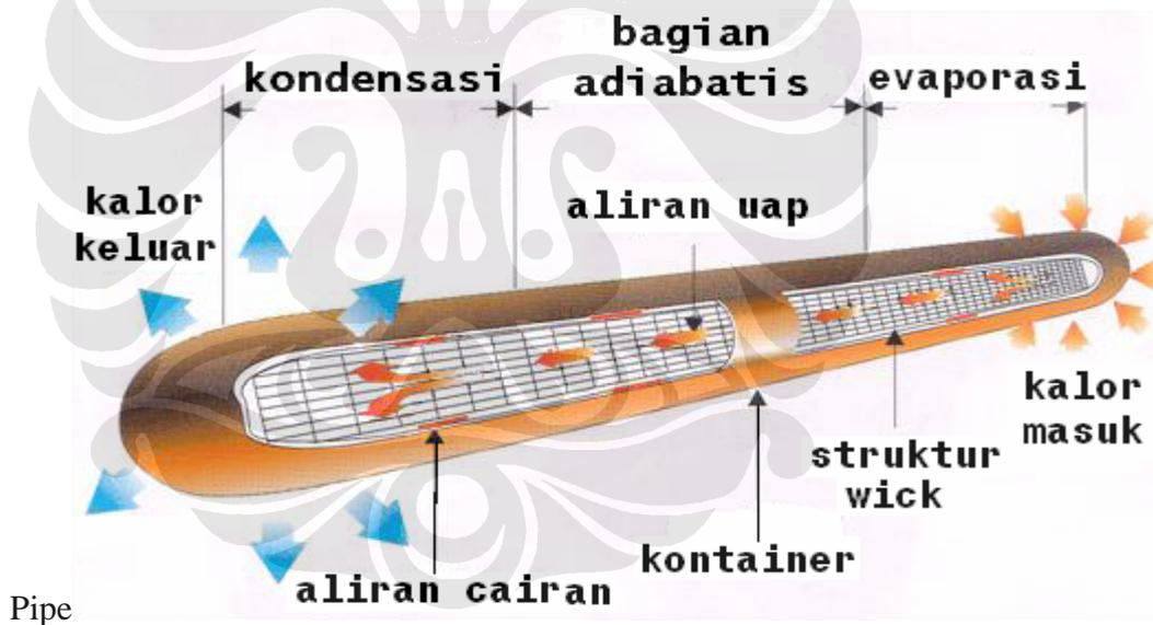
Gambar 2.3 Prinsip Kerja Heat Pipe
