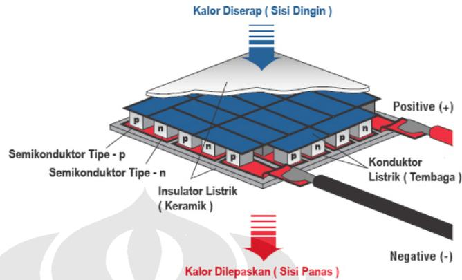
**Gambar 2.1** Skema aliran peltier ([www.melcor.com](http://www.melcor.com))
