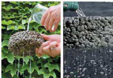
Gambar 2.16 *Porous concrete* (sumber: [www.porouspavement.com](http://www.porouspavement.com))
