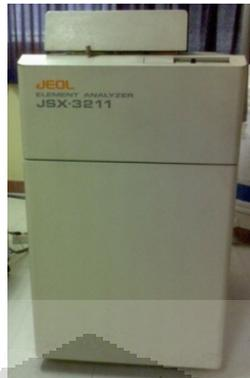
Gambar 3.2 XRF merek Jeol Element Analyzer JSX-3211
