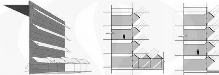
Gambar.28 Ilustrasi *Hybrid photovoltaics awning system*.
