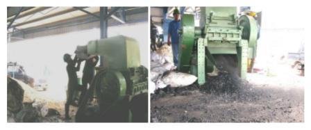
Gambar 26. Alat potong (*Crusher*) (Sumber: Indocement (a), 2008)
