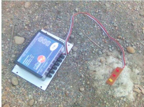
**Gambar 3.10** *Battery Charge Regulator (BCR)* <sup>[7]</sup>
