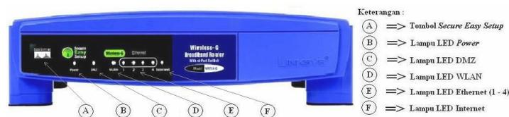
**Gambar 3.4.** *Tampak depan wireless router WRT54GL versi 1.1.*
