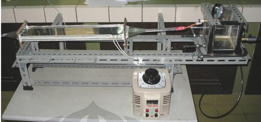
Gambar 3.4 Thermal Precipitator
