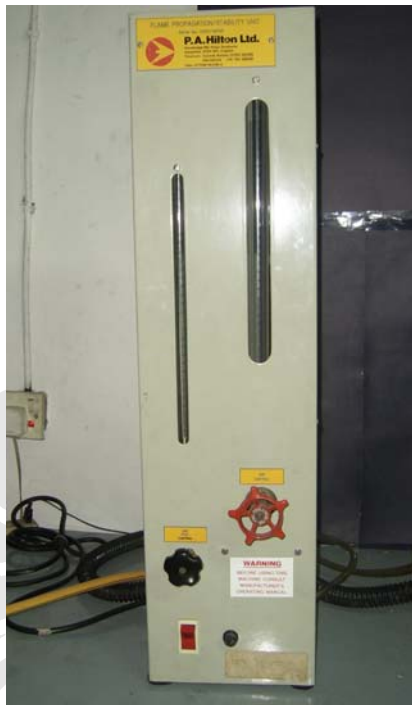
Rotameter Flame Propagation and Stability Unit P.A. Hilton Ltd. C551
