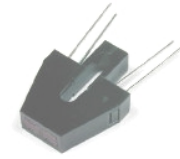
Gambar 3.5c. Sensor Proximity (Satu Kemasan)
