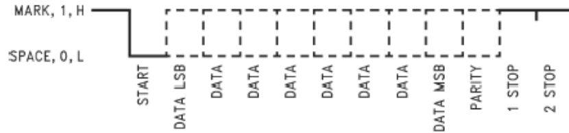
Gambar 2.7 Timing Format Asynchronous – UART
