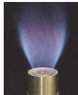
c. High-swirl flame generated by a vane swirler
