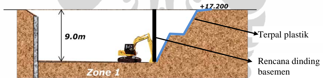
Gambar 6.8 Area Rawan Longsor/Erosi
