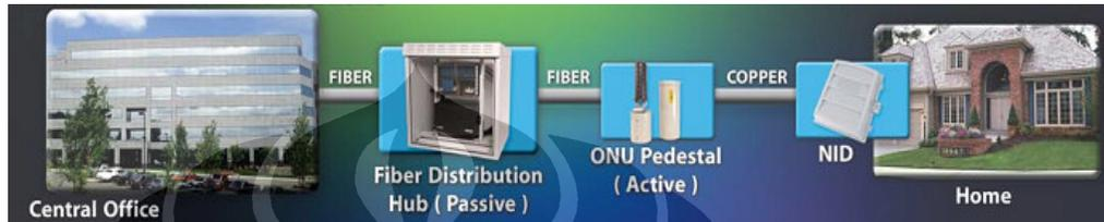
Gambar 2-8 : Jaringan FTTC (Fiber to the Curb) [8]
