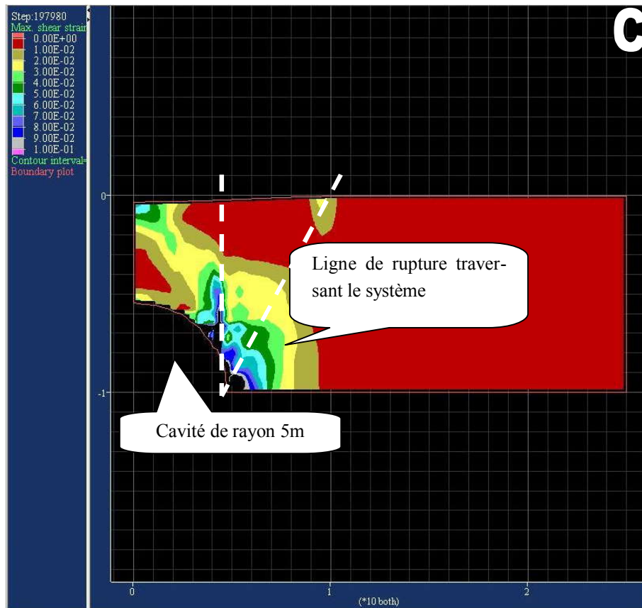
Figure 30 Development of \gamma^p during the creation of a cavity with total rupture (value obtained with r=5m ; C=80kPa )
