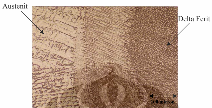
Gambar 4.1. Struktur Mikro WM Sampel 6, Ketebalan 3 mm Metoda GTAW
