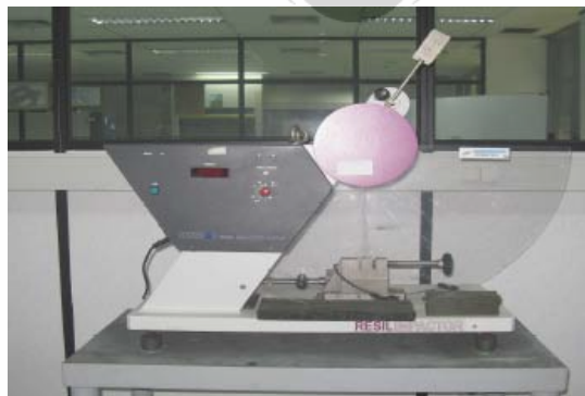
Gambar 3.11. Mesin Uji Impact CEAST Resil
