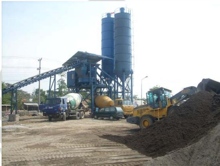
**Gambar 3.3** *Batching plant Wet Mix System*
