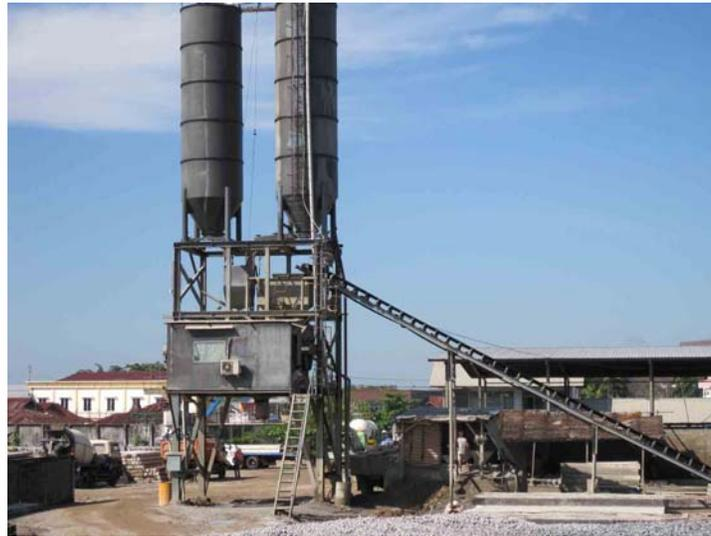
**Gambar 3.2 *Batching plant Dry Mix System***
