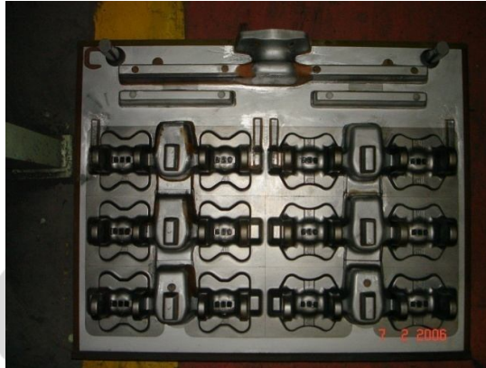
Gambar4. 6 Flange Yoke pattern (Sumber: PT. Y)
