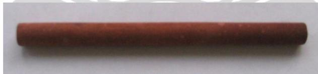
Gambar 3.8 Sampel *wick sintered powder*
