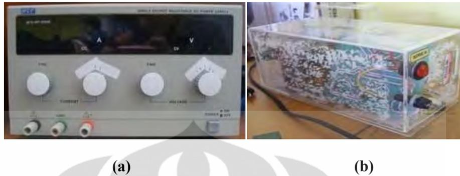
**Gambar 4. 8** (a)Power supply MCP tipe M10-SP-3020E, (b) Power supply custom
