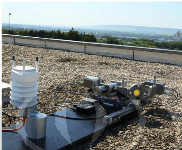
**Gambar 1.1** In Situ CO<sub>2</sub> Spectrometer
