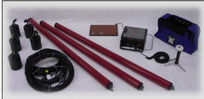
Gambar 4.2 1 Set alat pengukuran MT (Phoenix, 2008).
