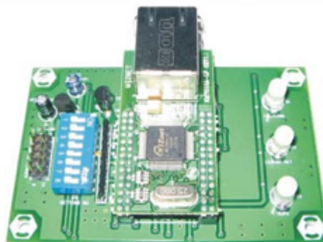
Gambar 3.9. TCP/IP Starter Kit [9]
