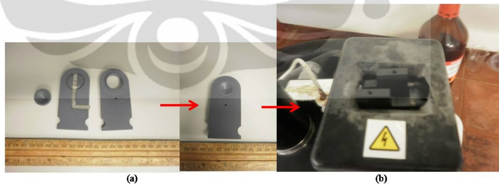
Gambar 3.67. (a) Sample holder . (b) Letak sample holder pada bak electropolishing .
