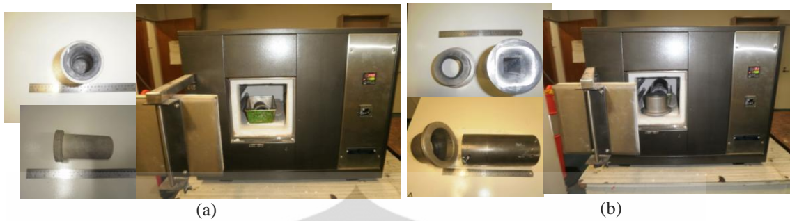
Gambar 3.15. (a) Proses preheating crucible . (b) Proses preheating cetakan.
