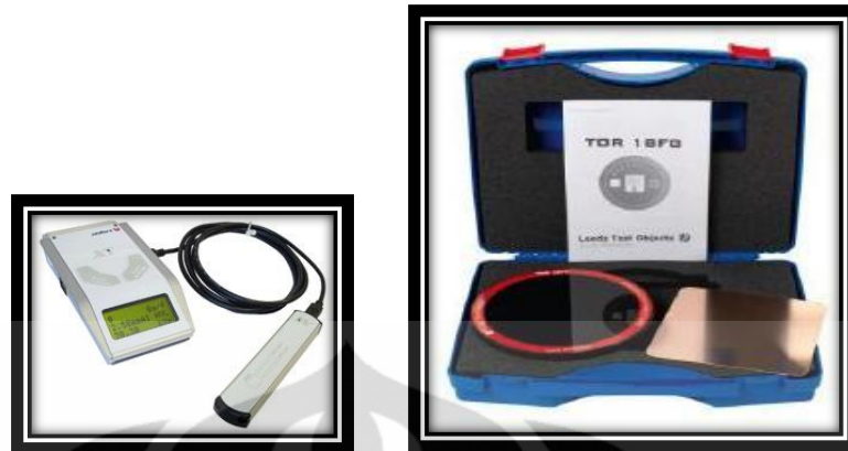
Gambar 3.3. Detektor unfors xi dan fantom leads TOR 18FG
