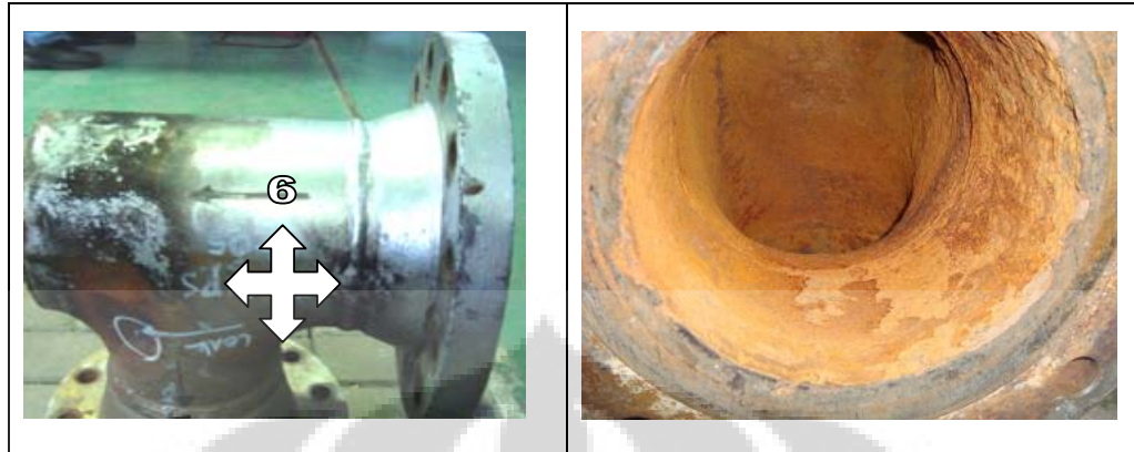
Gambar 4.7 Sampel pipa gagal A106 Gr.B
