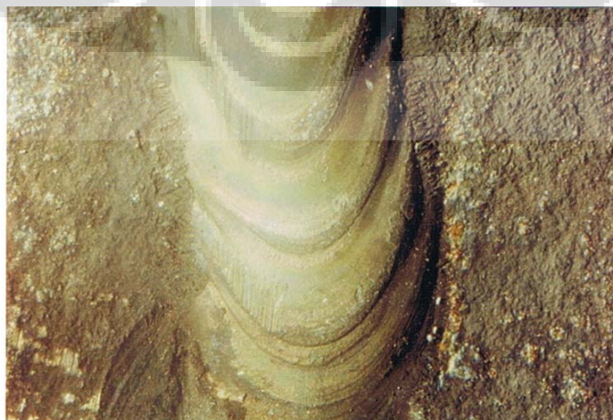
Gambar 4.2.1.2 Foto makro sample pendinginan air perbesaran 7x
