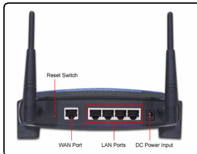
Gambar 3.2.b. Tampak Belakang Wireless Router Linksys WRT54GL
