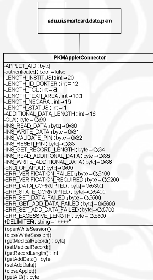
Gambar 3.3 Class Diagram Applet Connector
