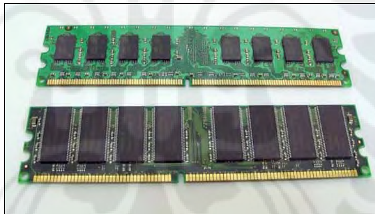
Gambar 2.5 DDR2 (atas) Vs DDR1 (bawah)
