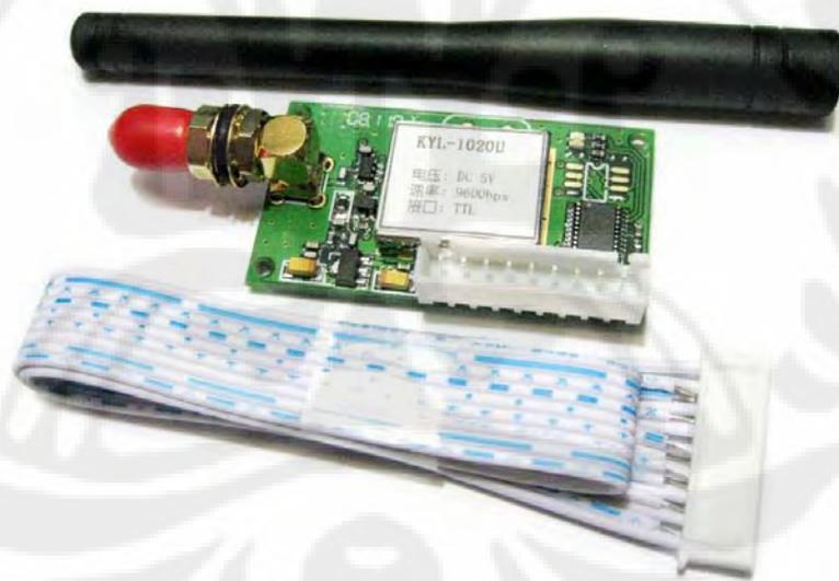
**Gambar 3.8** Gambar Rangkaian RF 1020U Data Transceiver [21].
