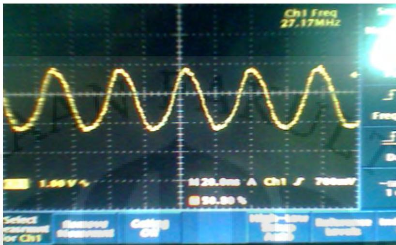
Gambar 4.6 Sinyal Masukan Rangkaian Superheterodyne channel 2
