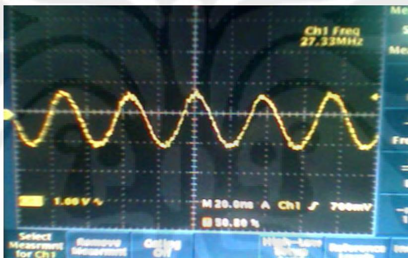
Gambar 4.7 Sinyal Masukan Rangkaian Superheterodyne channel 3
