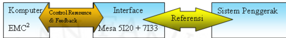
Gambar 2.1 Blok diagram pengendalian CNC
