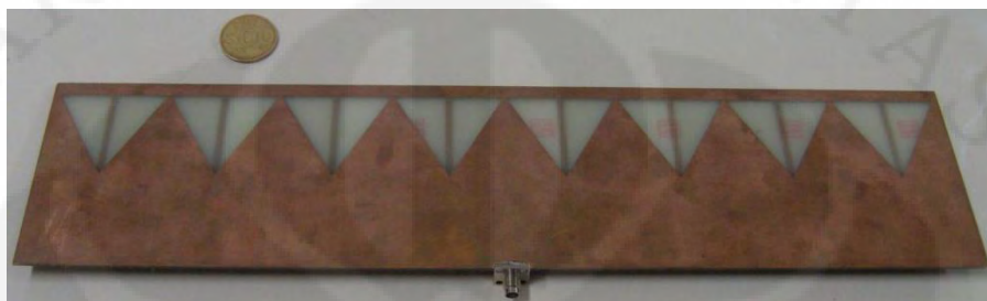
Gambar 4.3 Antena mikrostrip array 8-element
