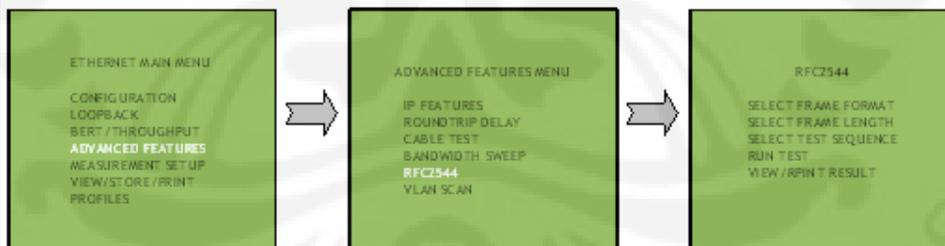
Sebelum [RUN TEST] terlebih dahulu tiga opsi yg ada ([SELECT FRAME FORMAT], [SELECT FRAME LENGTH] dan [SELECT TEST SEQUENCE]) kita setting.
