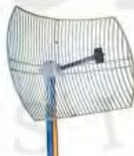
Gambar 2.8 Contoh Antena Directional [9]
