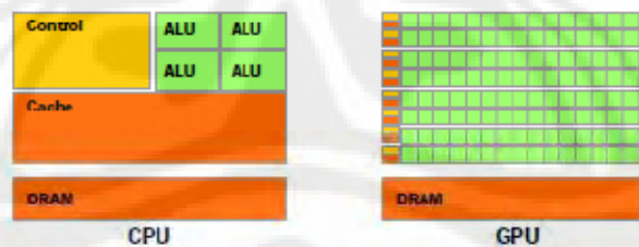
Gambar2. 6 Perbandingan CPU dan GPU (NVIDIA CUDA Programming Guide, 2009)
