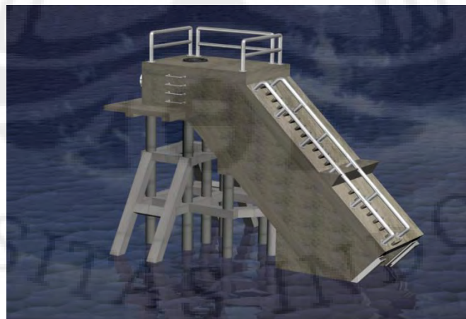
Gambar 3.4 Prototipe Sistem Oscillating Water Colum ( OWC ) [5]
