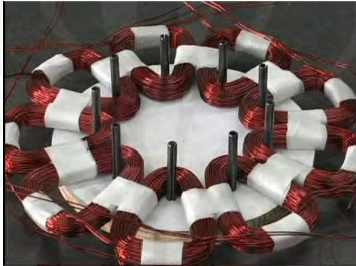
**Gambar 2.13** Stator Tanpa Inti
