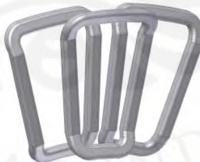
**Gambar 2.14** Overlapping Stator[4]
