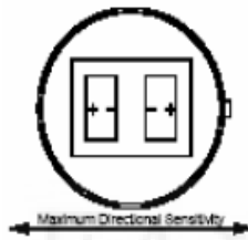
Gambar 2.3 – Sensor Pyro-electric (PIR) Elemen Ganda
