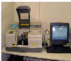
**Gambar. 3.2.** Gambar Spektrofotometer Inframerah ( *Fourier Transform Infra Red Spectrophotometer, FTIR*) Prestige 21.
