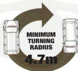
Gambar 4.5 Minimum turning radius mobil listrik
