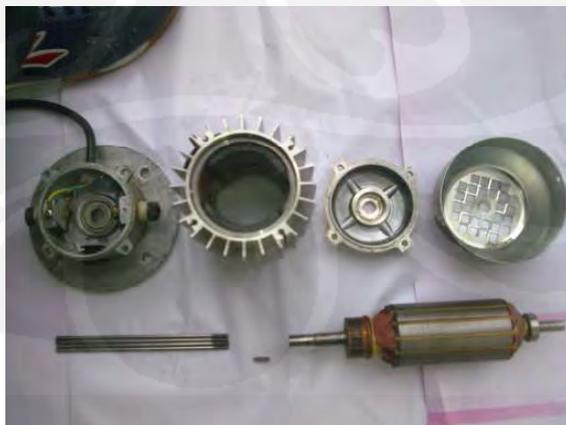
Gambar 3.10 Bagian-bagian motor dc magnet permanen
