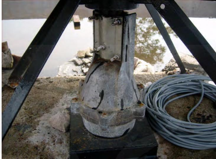
Gambar 2.13 T-2XX Tailtwister Rotator
