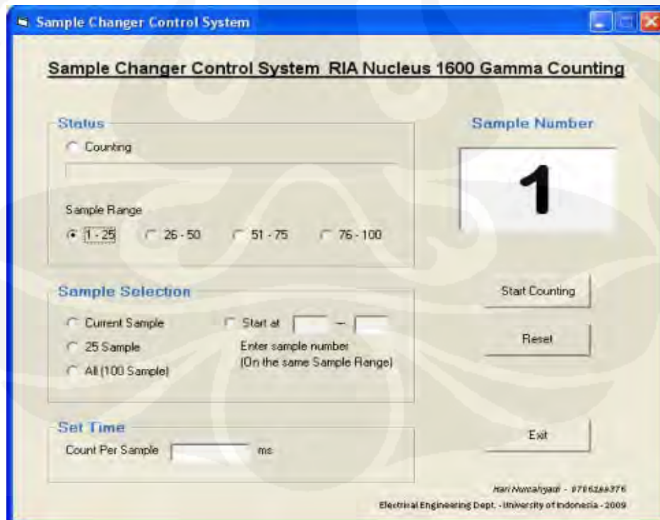
Gambar 4.6. Tampilan program sistem kontrol sample changer perangkat RIA Nucleus Model 1600 Gamma Counting
