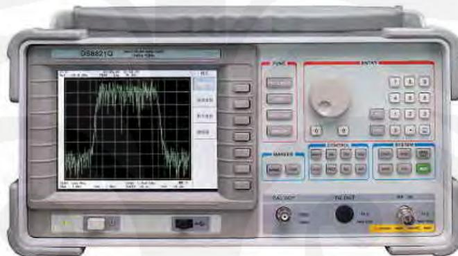
Gambar 2.14 *Spectrum Analyzer* (SPA) [6]
