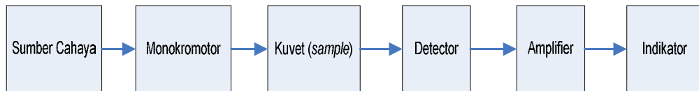
Gambar 2.9. Blok diagram spectrophotometer
