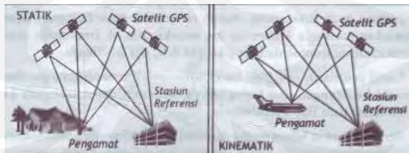
Gambar 2.5. Metode penentuan posisi differensial [1]
