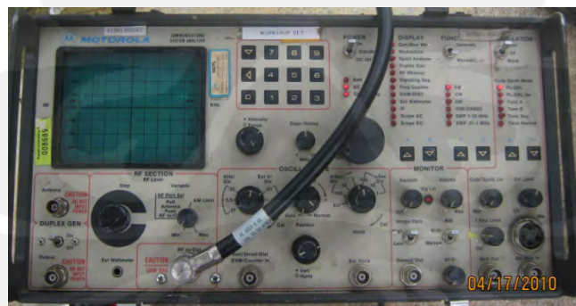
Gambar 3.16 Setup pengukuran Squelch
